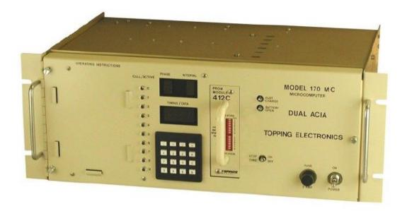
The Topping Electronics Model 170MC Controller is a solid-state microprocessor-based controller designed for use in harsh environments such as those found in traffic control applications. The 170MC is built with plug-in printed circuit modules and runs a Motorola 6802 microprocessor-based stored program providing logic control for traffic or other control applications. Operator interface with the controller is achieved by means of a front panel keypad and associated display indicators.
